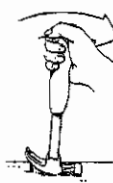
A claw hammer acts as a class-1 lever when used to pull a nail.
